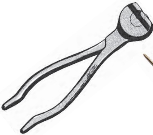
DIAMOND PIN AND WIRE CUTTER CUTS UP TO 2 mm WIRE
